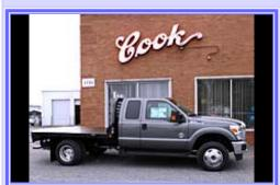
GOOSE BODY: Blue Ridge Mfg Rodeo Goose Body RD 9.5D, mounted on F350. Radius Tube Bulkhead with unobstructed rear window, 30000# Goose Neck Hitch, Asphalt undercoating of body, recessed lights and tag well. Body floor made of steel or aluminum.
