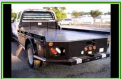
F450 CC 4x4, Blue Ridge Super Hauler 9.5' DRW; 96" Width. Trailer Plugs(2), Receiver Hitch, Goose neck hitch compartment w/ball.
