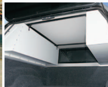
Toolboxes are securely fastened to roof rack framework
